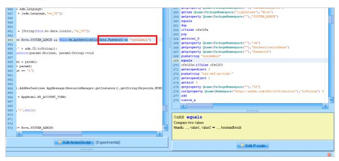
Figure 31. JPEXS decompiling index.swf showing default password
