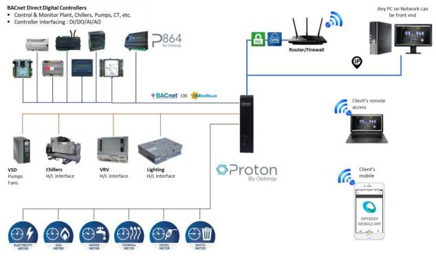
Figure 43. Optergy BMS typical network architecture
