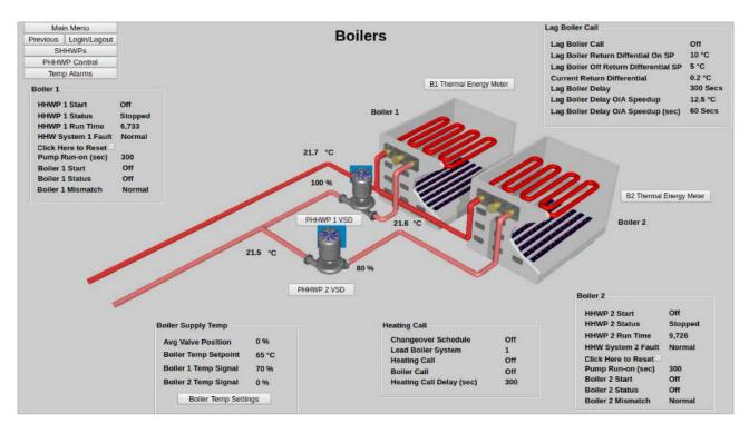
Figure 49. Optergy Boilers control interface
