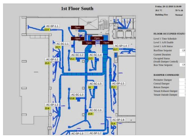
Figure 74. Optergy Floor Plan AC control
