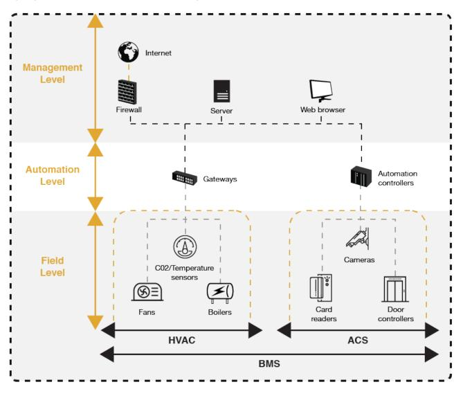
Figure 2. Relation between BMS components and systems
