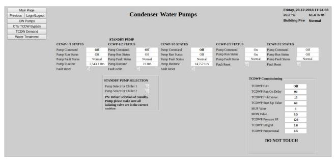
Figure 71. Optergy Condenser Water Pumps control
