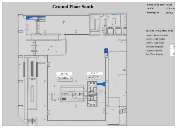
Figure 75. Optergy Floor Plan AC control
