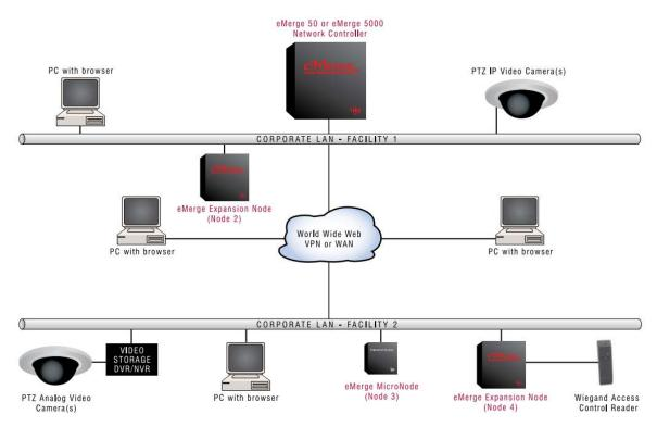
Figure 10. Linear eMerge network architecture [8]
