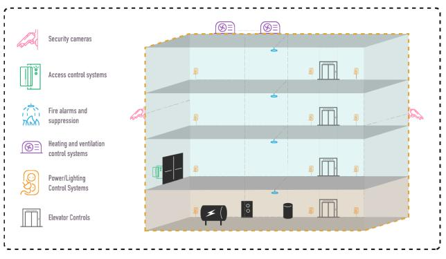
Figure 3. Examples of systems controlled by a BMS
